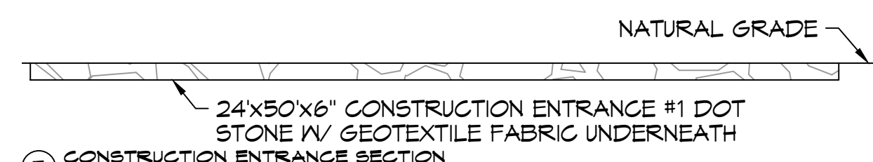
CONSTRUCTION ENTRANCE SECTION
