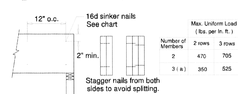
B12-A Side Loaded Connection Double & Triple 1-3/4" Versa-Lam® Nail Pattern
