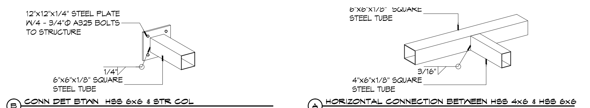
5 DETAILS SCALE: NTS OVERHEAD DOOR STRUCTURE DETAILS
