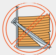
Nail Too Long
